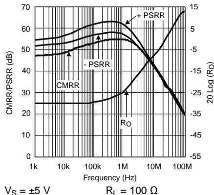
Figure 18. CMRR, PSRR,  $R_{OUT}$
