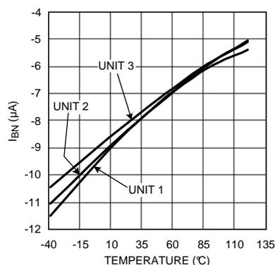
Figure 16. Non-Inverting Input Bias for 3 Representative Units
