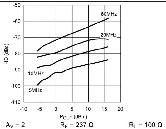
**Figure 12. HD<sub>2</sub> vs Output Power (Across 100  $\Omega$ ) (SOIC Package)**
