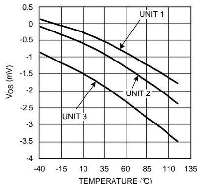
Figure 14. Input Offset for 3 Representative Units
