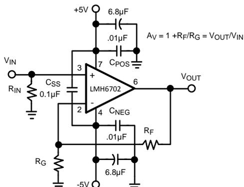
Figure 24. Recommended Non-Inverting Gain Circuit
