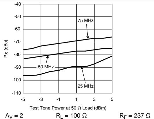
**Figure 10. 2 Tone 3rd Order Spurious Level (SOIC Package)**
