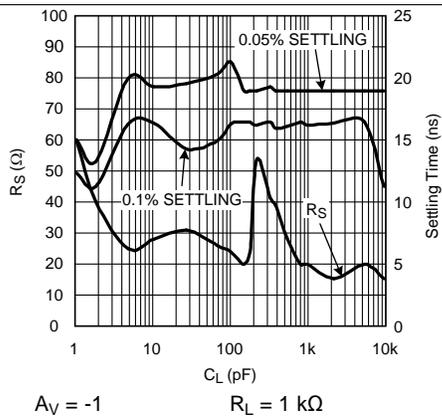
**Figure 11.  $R_S$  and Settling Time vs  $C_L$**
