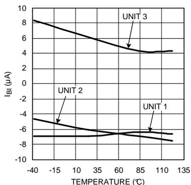
Figure 15. Inverting Input Bias for 3 Representative Units
