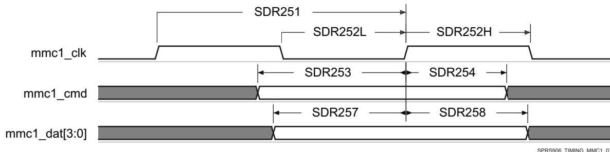
Figure 7-61. MMC/SD/SDIO in - High Speed SDR25 - Receiver Mode
