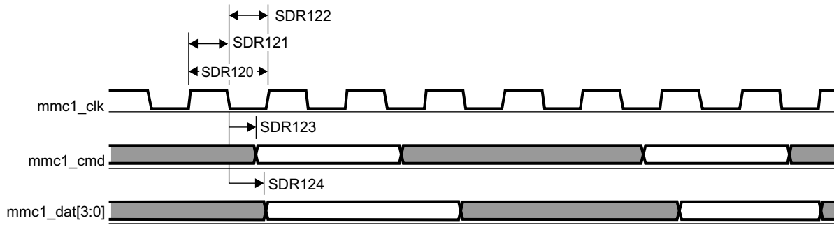
Figure 7-60. MMC/SD/SDIO in - High Speed SDR12 - Transmitter Mode
