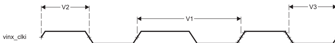
Figure 7-4. Video Input Ports clock signal
