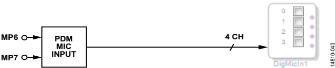
Figure 45. PDM Microphone Input Mapping to DSP in SigmaStudio
