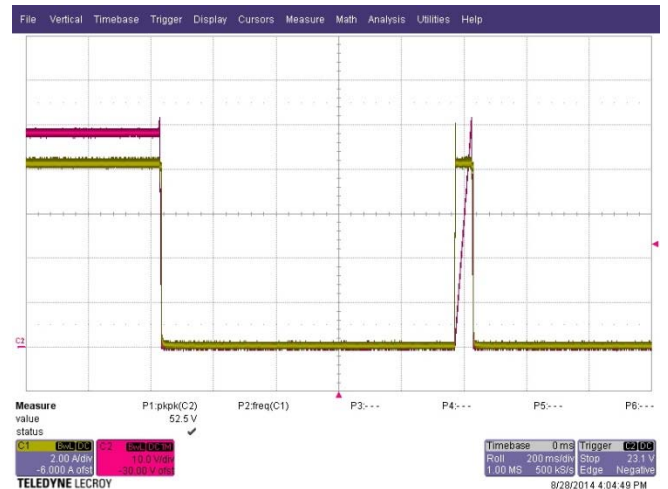
Figure 31. Overvoltage Shutdown and Retry; Red Trace = Output Voltage, 10 V/div, 200 ms/div; Yellow Trace = Secondary Current, 2 A/div
