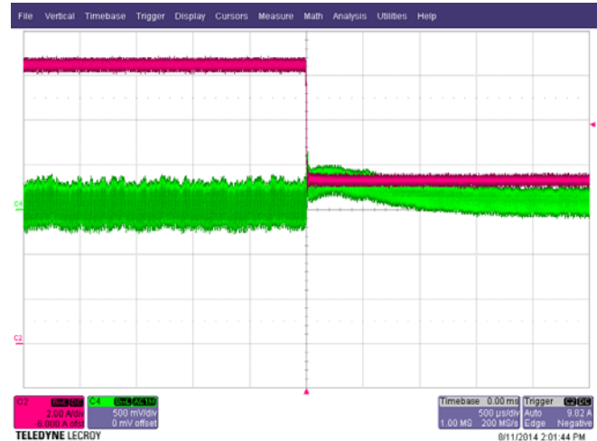
Figure 35. Dynamic Performance 600 W to 300 W, 385 V dc Input; Green Trace = AC-Coupled Output Voltage, 500 mV/div, 500 \mu s/div; Red Trace = Load Current 2 A/div
