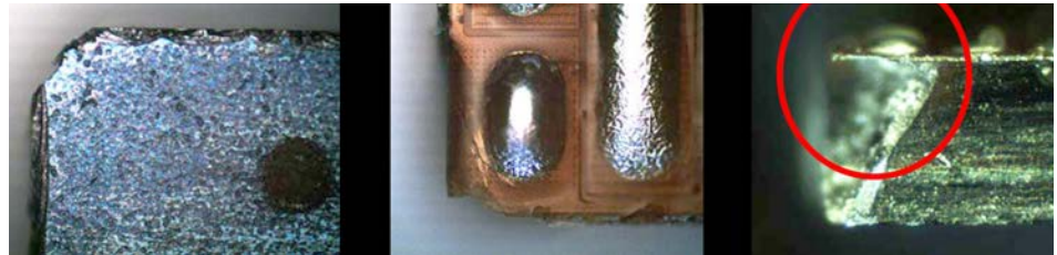
Fig 4b: Visual reject part shown in pictures above – EPC1001 part with severe corner chip. Back side chip extends all the way through the chip. Die was still functioning in application. Die is shown post dismount from PCB board.
