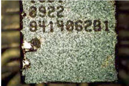
Fig 4c: EPC1001 part (above) passed 1000 Cycle TC -40°C to 125°C. Die width ~1900µm Back side chip >250µm
