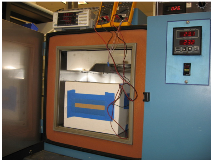
Figure 13 – Thermal Chamber Set-up Showing Box Used to Prevent Airflow Over UUT.
