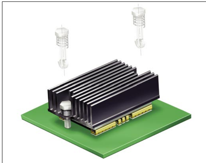
Figure 2 Mounting a heat sink to the BCM increases the effective surface area and lowers R\theta_{CA} .
