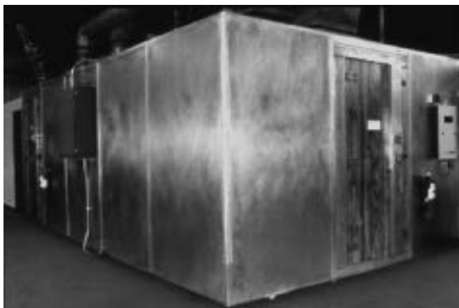
The Curtis screen room provides complete RFI isolation for equipment under test and the test instrumentation.
