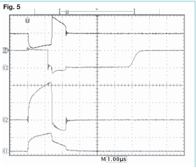
contributes a measurement error to trace R2. Although a low inductance shunt is used, it does have 10 nH of inductance which adds a voltage drop not representative of the current value. In this case, this inductance provides a 1 volt drop at a current rise rate of 100 A/μs. This can be seen at the turn on of the MOSFET where the voltage across the shunt instantaneously jumps to 1 volt, and during the turn off phase when the voltage instantaneously goes negative.
