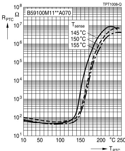
**Sensors****Motor protection, single sensors****M1100****Characteristics (typical)**
