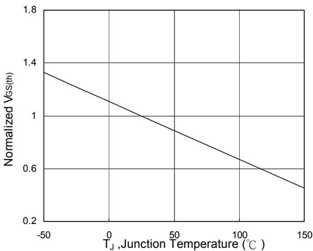
**Fig.5 Normalized V<sub>GS(th)</sub> vs. T<sub>J</sub>**
