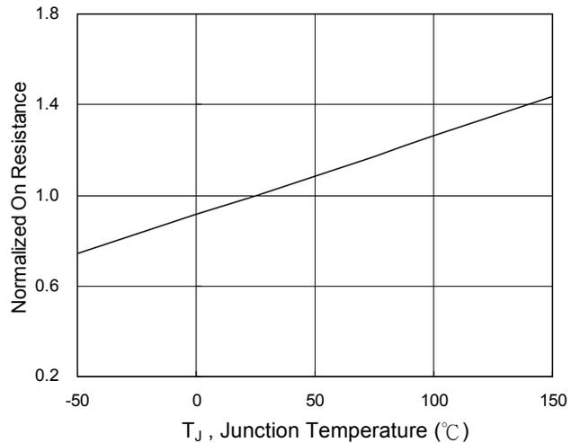
**Fig.6 Normalized R<sub>DSON</sub> vs. T<sub>J</sub>**
