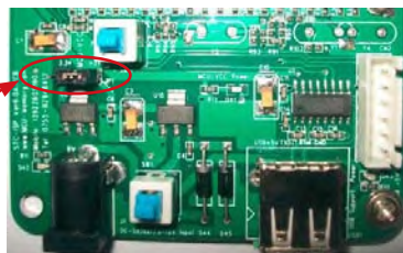
单片机电源电压的选择跳线短接MCU-VCC和5V电源管脚
