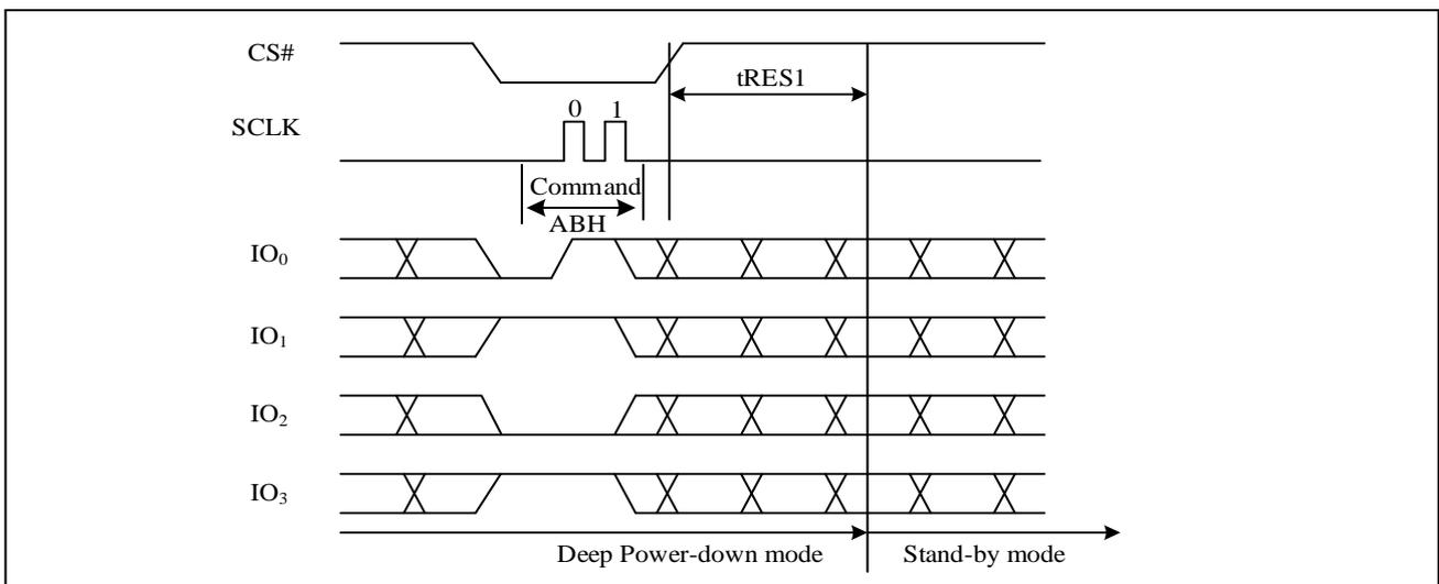
Figure23. Release Power-Down/Read Device ID Sequence Diagram
