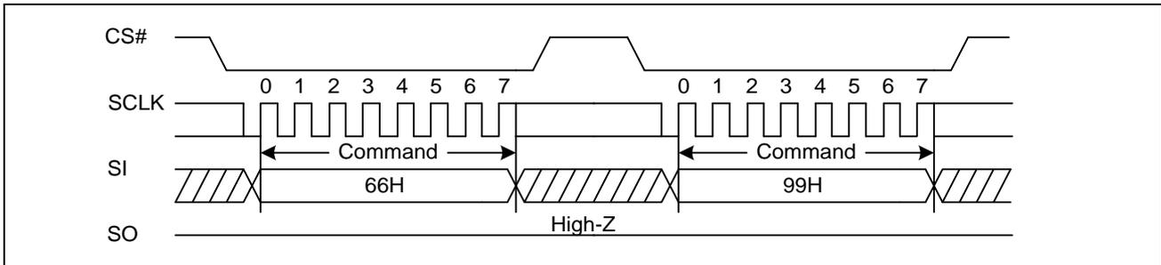
**Figure39. Enable Reset and Reset command Sequence Diagram (QPI)**
