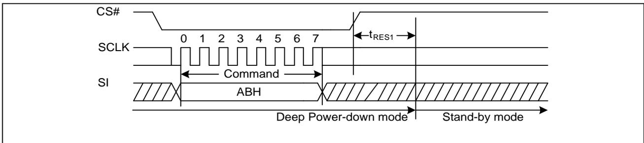
**Figure22a. Release Power-Down Sequence Diagram (QPI)**
