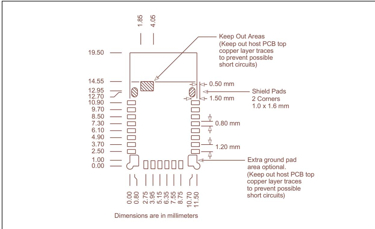
**FIGURE 4-3: RN4020 MODULE MOUNTING DETAILS**
