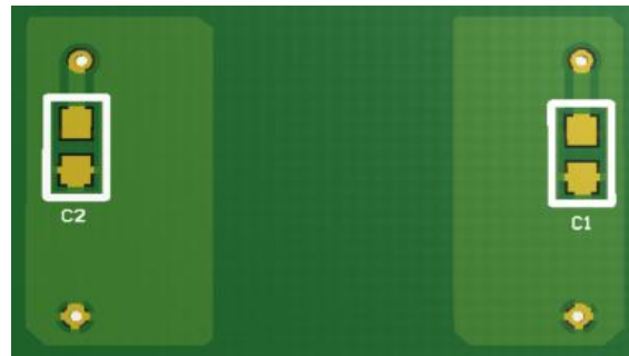
Figure 8.2 Recommended PCB Layout — Bottom Layer
