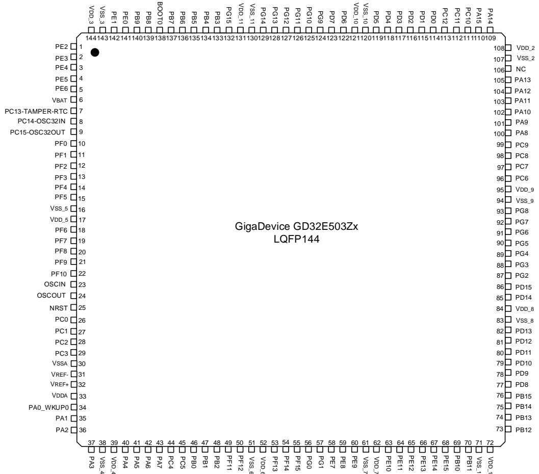
Figure 2-2. GD32E503Zx LQFP144 pinouts
